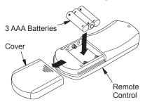
Figure 34 - Installing Batteries in Remote Control
